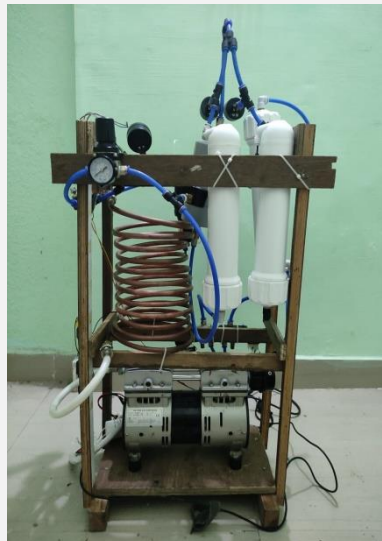
PSA Oxygen Concentrator
