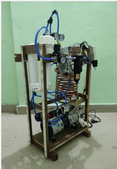
PSA Oxygen Concentrator
